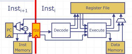
Inst<sub>i+1</sub> is not known until Inst<sub>i</sub> is at least decoded. So which instruction should be fetched?
